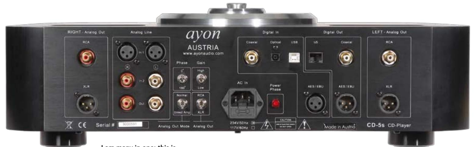
**I am many in one: this is definitely not how the back of a pure CD player looks like. With its CD-5s, Ayon offers a complete digital converter board – plus analogue cinch and XLR inputs.**
